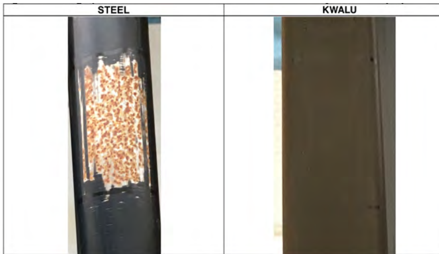
Figure 4: Photographs of chairs after razor and steel wool and 13 days of bleach preparation
